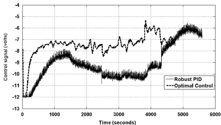
Figure 14. Optimal control signal versus robust PID signal.
