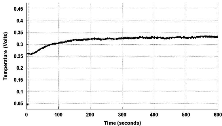
Figure 2. Step response of the process.
