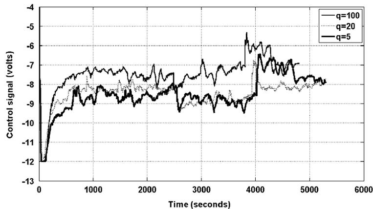
Figure 12. Implemented optimal control signals with the composed Simpson's rule.
