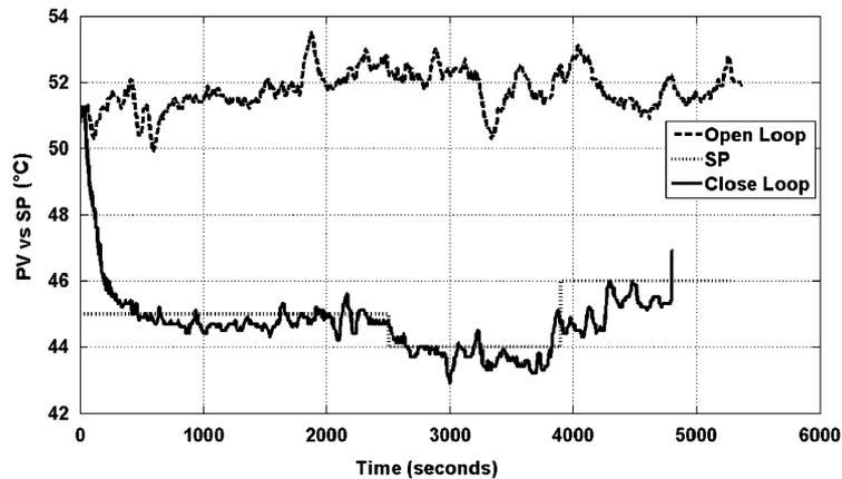
Figure 9. PV in open and closed loop.
