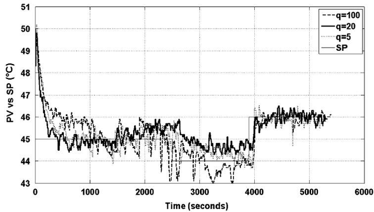
Figure 16. Comparison of PV responses with optimal control law approximated by composed Trapezoidal rule.
