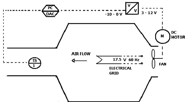
Figure 1. Instrumentation diagram.
